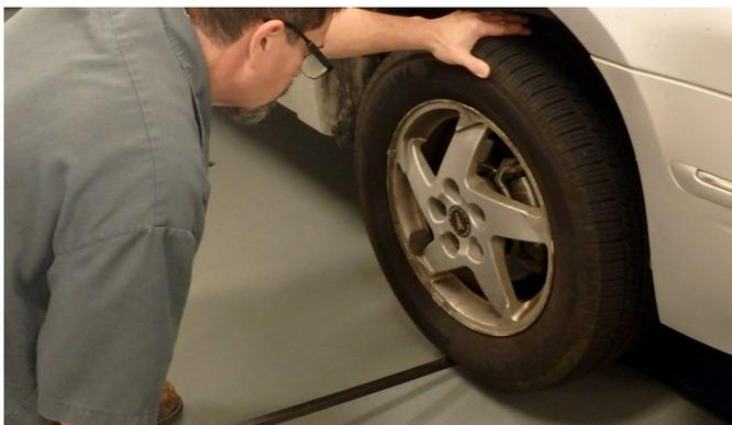
**Step 5** – If using a dial indicator to check axial and radial looseness, attach the dial indicator and measure axial looseness by using a pry bar to lift the weight off the unloaded tire and wheel assembly.
