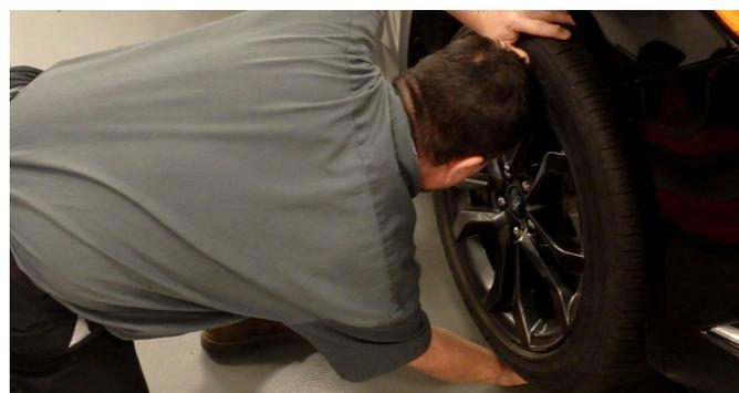
**Step 4** – Check for axial looseness by using a pry bar to lift up the tire.
