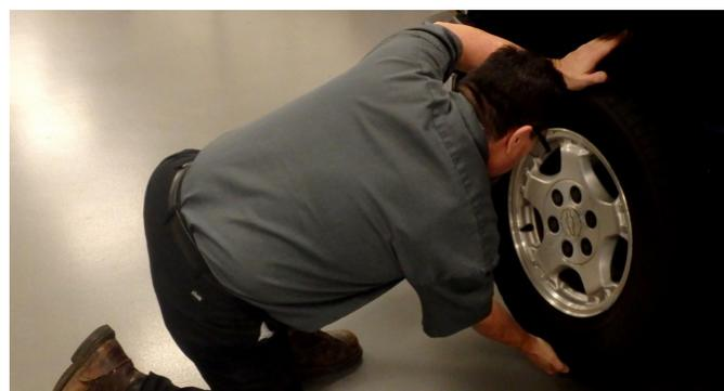
**Step 3** – To inspect the ball joint on a MacPherson strut suspension for radial looseness, lift the vehicle off the ground and move the tire in and out.
